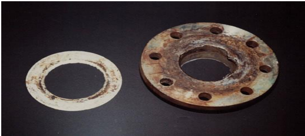
Gambar 5.5 korosi Celah ( Crevice Corrosion )
